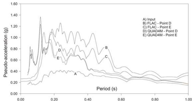
Fig.11. Comparison between numerical spectra calculated by FLAC and QUAD4M.
