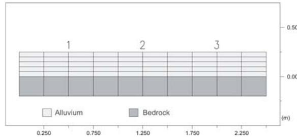
Fig. 4. Simplified testing section utilized to compare FLAC and QUAD4M results obtained at the three selected monitored points labeled 1, 2, 3.
