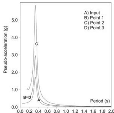
Fig. 8. FLAC spectra regarding equation (6); responses of points 1 and 3 are identical.
